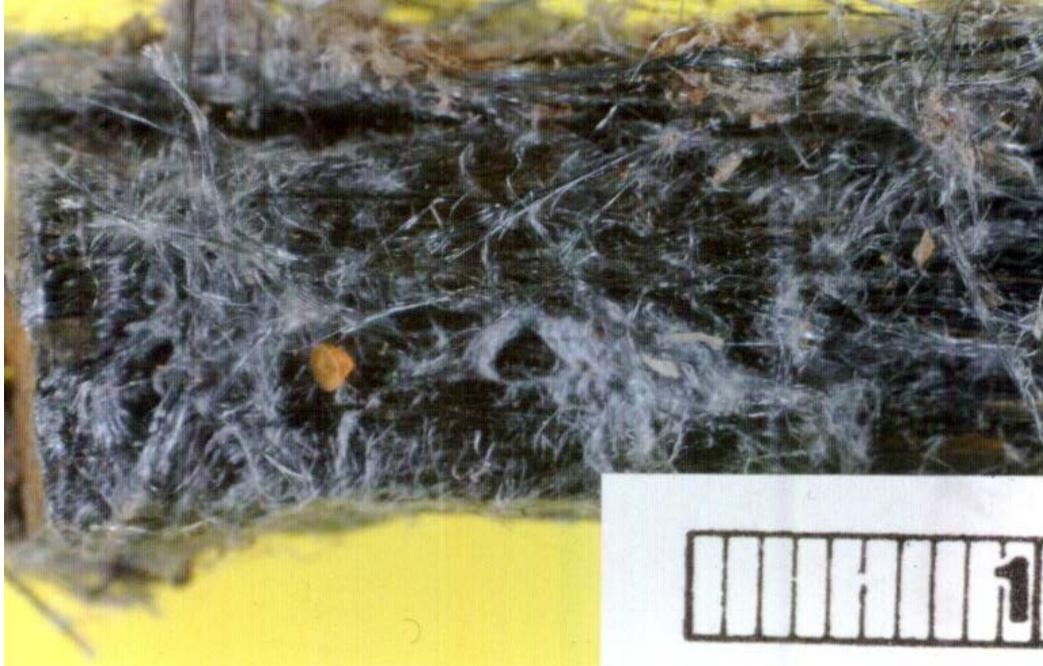
**Blue asbestos** showing the fibrous nature of the mineral. The ruler is 1 cm.
