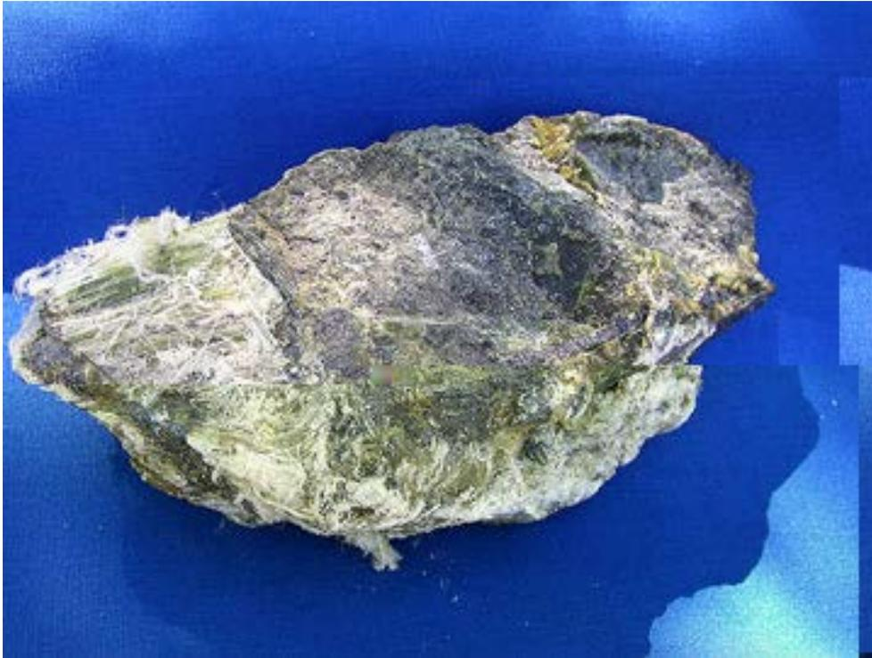
**Chrysotile or white asbestos** is the most commonly encountered form of asbestos.
